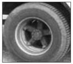
cracks or distortion around the bolt holes. "Bud" or "Dish" wheels should have space between them and free of debris. The hub oil seals, axle seals and wheel bearing seals should not be leaking.
